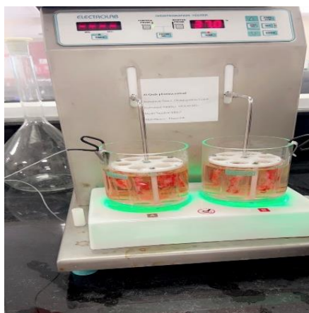
Figure 15: Residence time Determination by Using Disintegration Apparatus at 37 \pm 1^\circ\text{C} .
